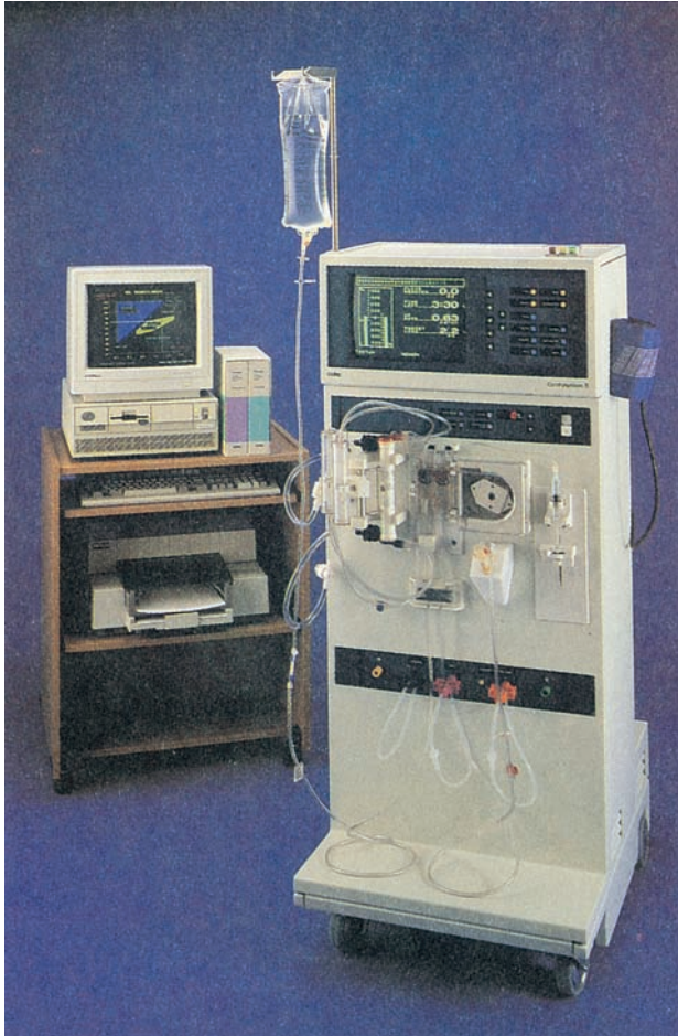
FIGURE 7-64 A hemodialysis machine helps remove waste products from the blood when the kidneys are not functioning correctly.
