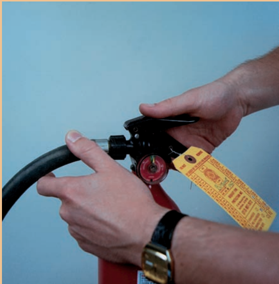
FIGURE 13-14C Aim the nozzle at the near edge of the fire, and push the handle to discharge the extinguisher.
