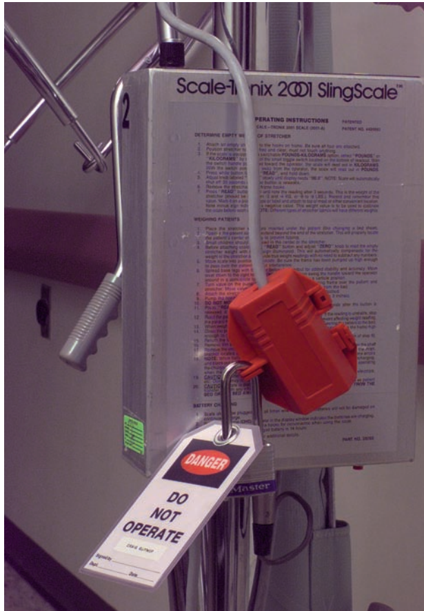
FIGURE 13-5 Some facilities use a lockout tag system for damaged equipment to prevent anyone from using the equipment.
