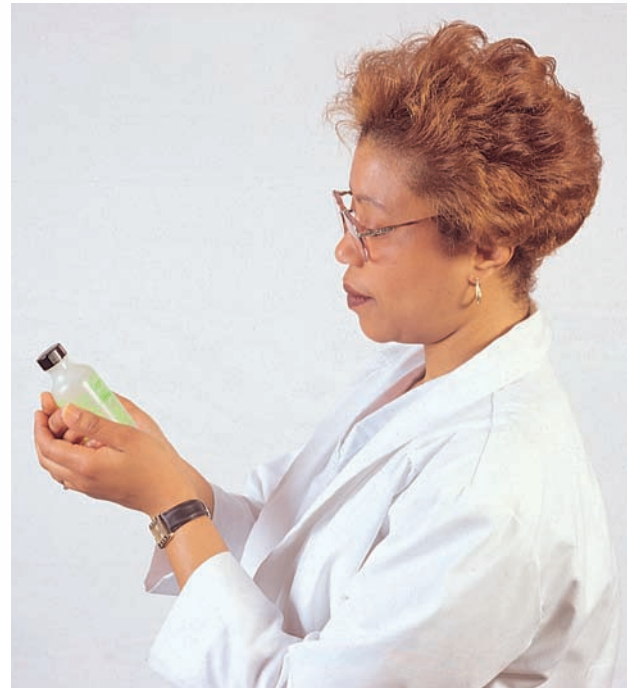
FIGURE 13-6 Read the label on a solution bottle at least three times to be sure you have the correct solution.
