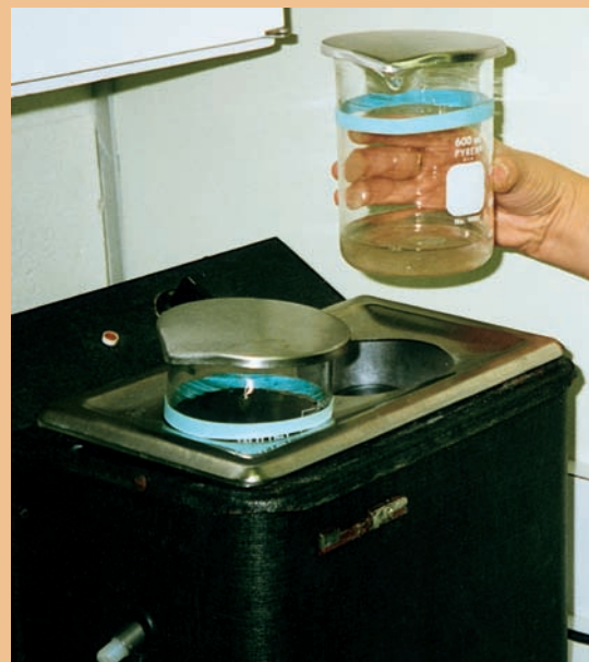
FIGURE 14-33B Glass beakers can be used to clean smaller items in an ultrasonic unit.
