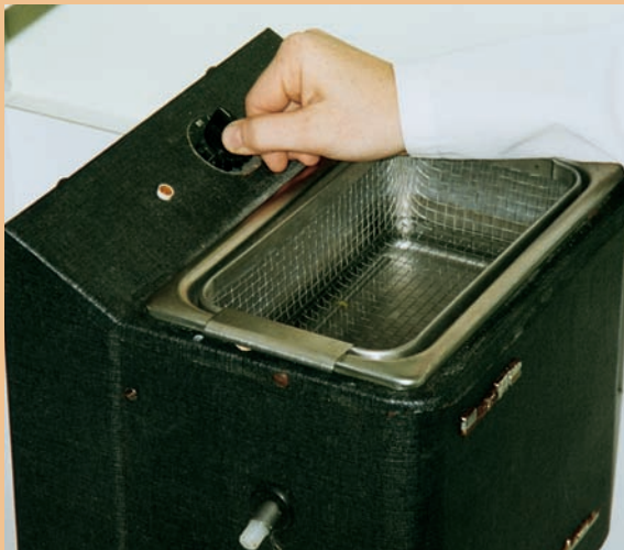
FIGURE 14-33A The auxiliary basket can be used to clean larger items in an ultrasonic unit.
