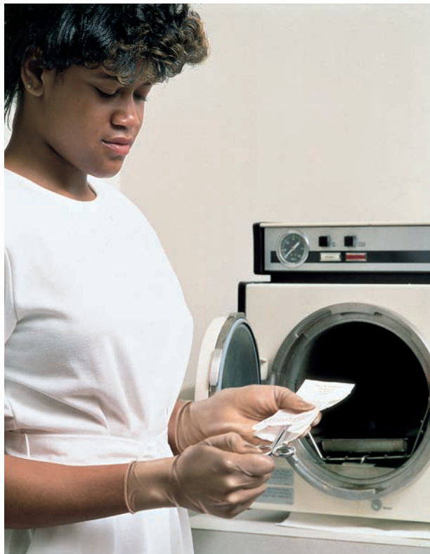
FIGURE 14-23 Special plastic or paper autoclave bags can be used to sterilize instruments.
