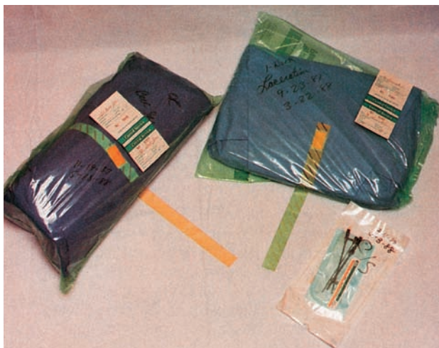
FIGURE 14-24 Autoclave indicators change color to show that sterilization has occurred. The strips below each package show how the indicators looked before sterilization.
