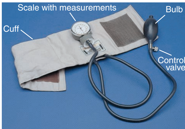
FIGURE 15-27A The gauge on an aneroid sphygmomanometer does not contain a column of mercury.
