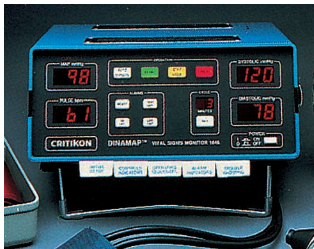
FIGURE 15-28 Electronic sphygmomanometers provide a digital display of blood pressure and pulse readings.
