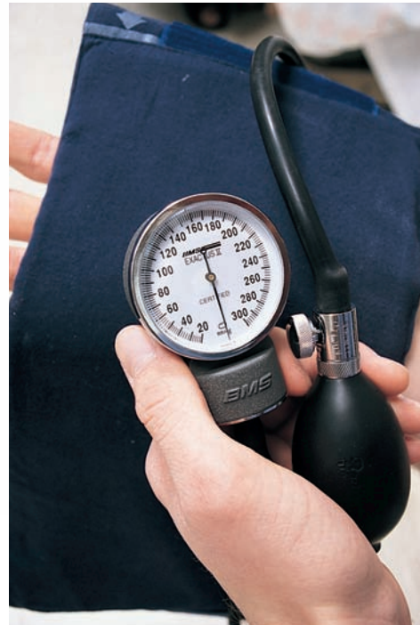
FIGURE 15-27B If the needle is not on zero when the aneroid cuff is deflated, the sphygmomanometer should not be used until it is recalibrated.
