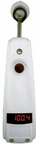
FIGURE 15-6 Temporal scanning thermometers measure the temperature in the temporal artery of the forehead. (Courtesy of Exergen Corporation, Watertown, MA)
