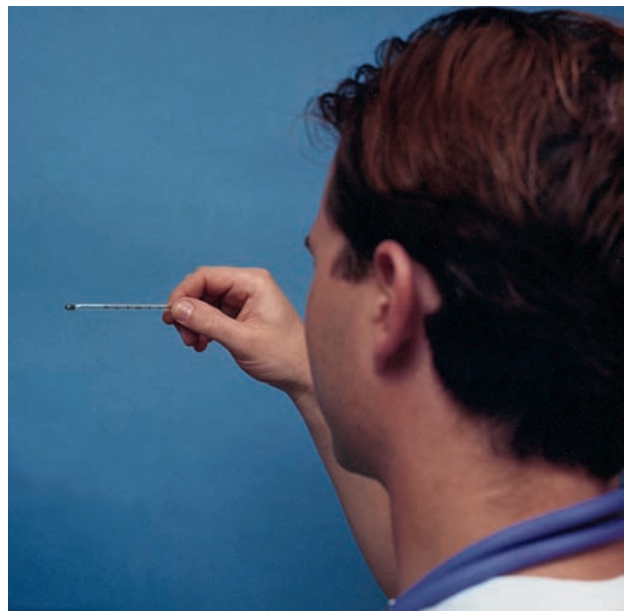
FIGURE 15-8 A clinical thermometer must be held at eye level to find the solid column of mercury or alcohol.
